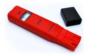
The pHep is an electronic pH measurement and display device. It is equipped with a digital display, two potentiometers for calibration, a pH electrode and a reference electrode. The compact housing design allows fast pH measurements in laboratories and in production sites.
