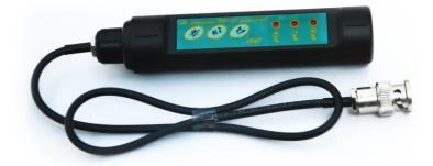
The CSP-101 is a pH simulator used for controlling and calibrating of the accuracy of pH measuring devices. It enables a fast and easy verification of the functional capability of the pH measuring device. The simulator delivers an output signal which is similarly created by an ideal pH electrode at 20  $^{\circ}$ C.
