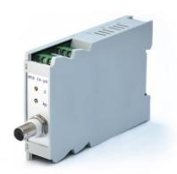
The MUH04-pH is a pH transmitter with a high-impedance, galvanically isolated pH input. The asymmetry potential and slope of the pH electrode can be precisely adjusted by two potentiometer on the front of the device. The connection of the pH electrode is established by a BNC connector or by screw terminals. The housing is suitable for rail mounting according to DIN EN 60715. The power supply and signal output terminals are connected by screw terminals.
