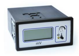
The MR48mVD is a high-resolution redox measurement, display and control device. It is equipped with a digital display and a limit switch. The desired value can be adjusted by a potentiometer. An LED indicates the limit switch condition. The limit can be displayed by using an additional button. The compact design according to DIN IEC 61554 is made of flame-retardant noryl and designed for panel mounting. The device is connected via screw-type connectors on the back side.
