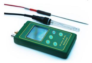
The CP-411 is a high-resolution measuring and display device for measuring pH, redox potential and temperature. It is equipped with an easy-to-read display. The device is connected via screw-type connectors on top.
