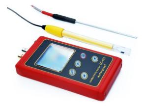
The CC-411 is a high-resolution measuring and display device for conductivity and temperature. It is equipped with an easy-to-read display. The device is connected via screw-type connectors located on top.
