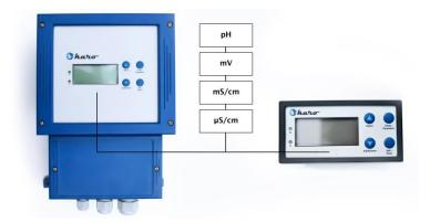
The karo is a high-resolution measurement and control device for measuring pH, redox and conductivity. The compact housing structure according to DIN IEC 61554 made of flame-retardant noryl is designed for panel mounting. The device is connected via screw-type connectors on the back side.
